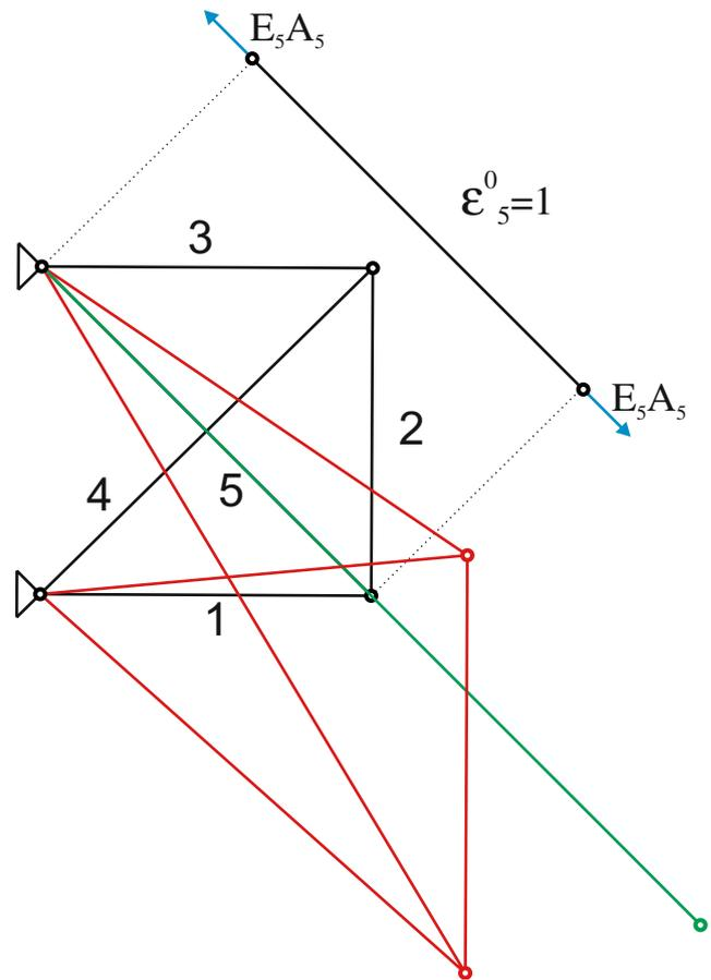
Fig. 2 Influence of the unit distortion applied in chosen location
