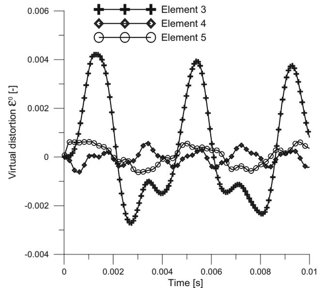
**Fig. 9** Virtual distortions modeling assumed stiffness modifications
