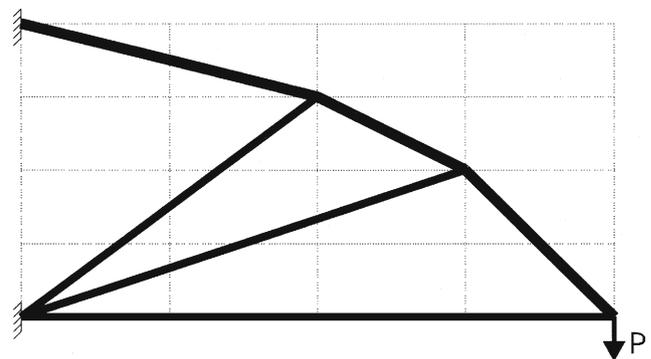
**Fig. 5** First optimal topology for the 136-element ground structure
