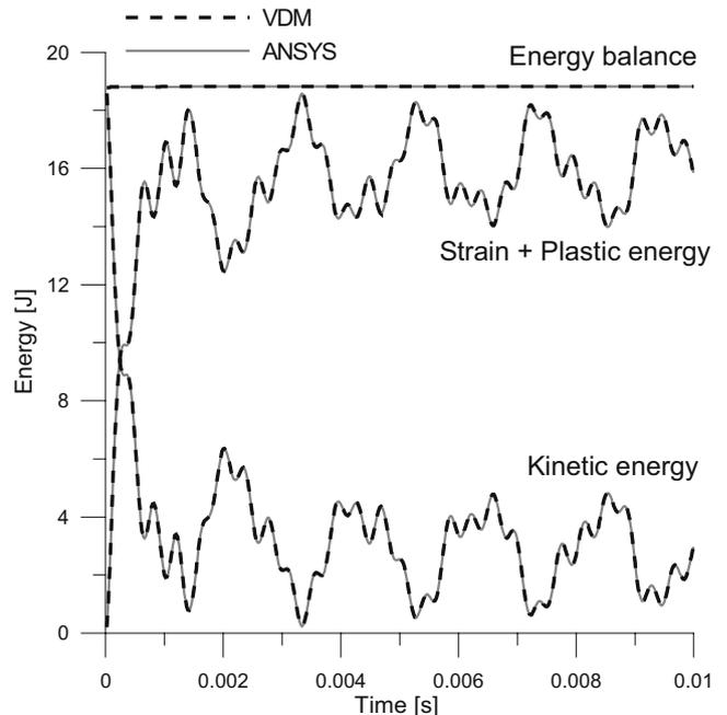
**Fig. 12** Energy balance of the five-element truss
