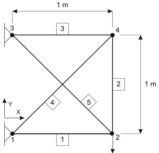
Fig. 4 Five-element truss structure for testing VDM algorithms
