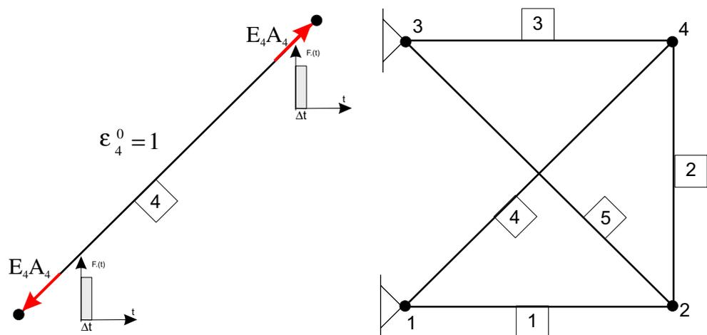
**Fig. 8** Impulse virtual distortion at a node, showing the process of matrices  $B^p$  and  $D^p$  composition
