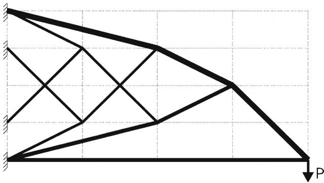
**Fig. 6** Second optimal topology for the 136-element ground structure
